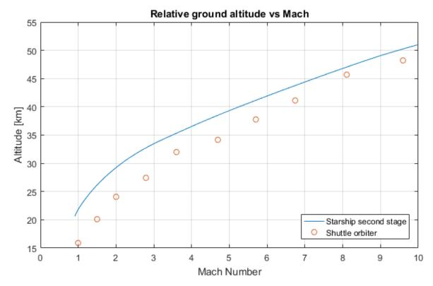
Figure 7: Approximate comparison of second stage RTLS descent trajectory and Shuttle Orbiter
