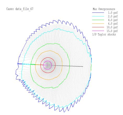
Figure 3: PCBoom v6.6 Pressure contours and isopemps for the 268 degree Super Heavy RTLS trajectory
