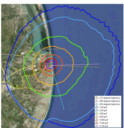
Figure 4: PCBoom v6.6 Pressure contours for a nominal Super Heavy RTLS at 1, 2, 4, 6, 10, 15, and 21 psf, overlayed with a map. The white line indicates the supersonic portion of the Super Heavy trajectory.
