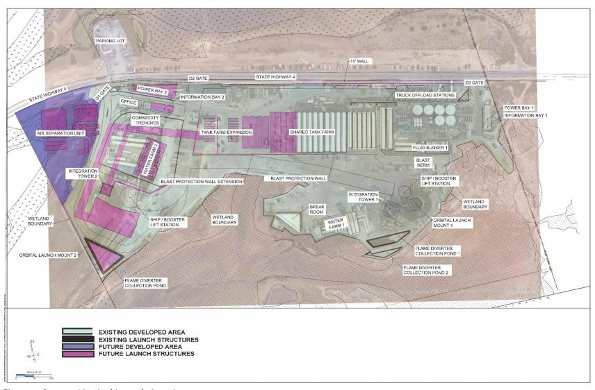
Figure 1 Current Vertical Launch Area Layout
