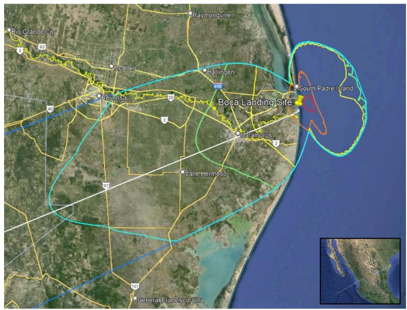
Figure 9: Starship second stage RTLS with 68 degree heading, augmented PCBoom + 1122 Ground Track Prediction (ZOOM)
