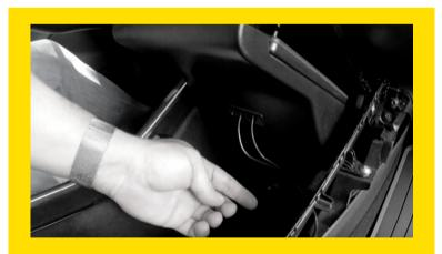
To get the cables to go under the trim, you will need to cut down/drill a small opening for the cable to pass through near the very front of the trim.
