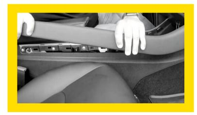
Once the cables are in place, make sure the Jeda Wireless Pad is connected and working properly. After verifying this, replace the plastic bumpers, metal trim, screws, and original plastic trim. Happy charging.
